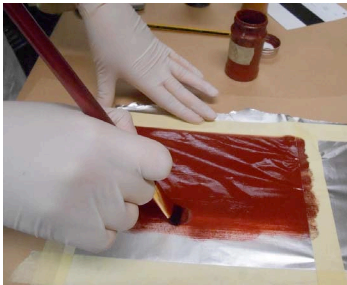
Picture 9. Samples for measuring elasticity (Photo: Barbara Škander, May 2014)
