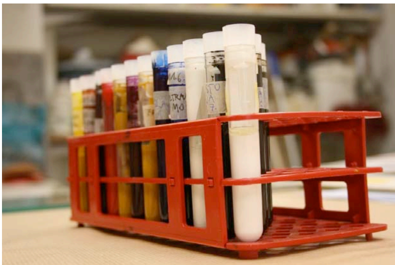
Picture 12. Samples for measuring paints' stability (Photo: Nina Dorič Majdič, August 2014)
