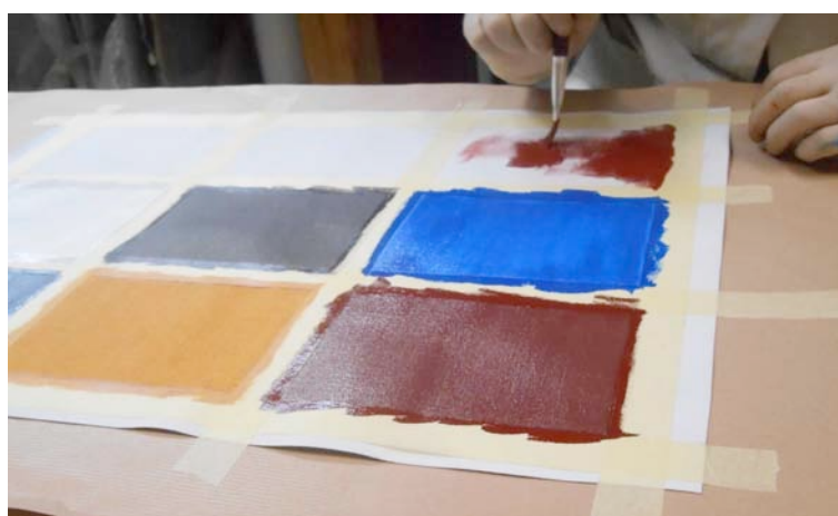
Picture 7. Preparation of samples for measuring effects of accelerated aging and UV light exposure (Photo: Nina Dorič Majdič, April 2014)
