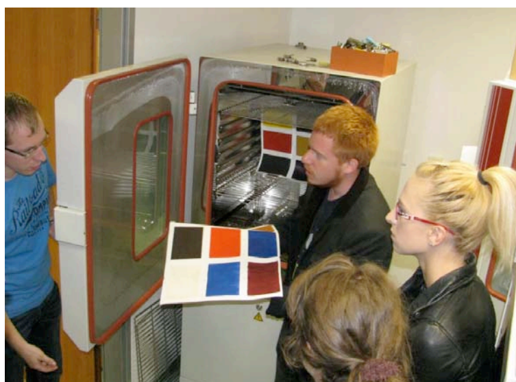
Picture 8. Results of samples after 63 days in accelerating age chamber (Photo: Nina Dorič Majdič, June 2014)
